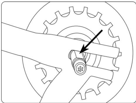
Place the Smart Wheel into the rear fork. The axle is flat on two sides in order to prevent it from rotating in place.
