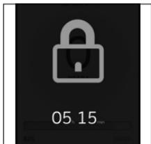
While the Smart Wheel is locked, a large lock appears on the screen with the estimated time the Smart Wheel can stay locked.
