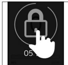
To unlock the Smart Wheel, hold the lock icon until the ring around the lock is completed.
