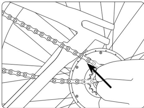
Turn the Smart Wheel so that the sprocket is on the same side as the chain of your bike.
