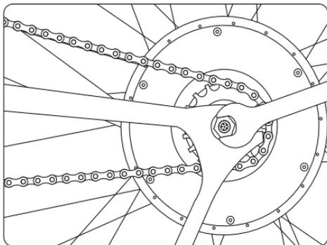
Loosely attach the first M12 axle knot. Loosely attach the second M12 axle knot on the other side.
