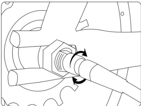
Gently turn the silver ring and screw the charger into the socket on the Smart Wheel.
