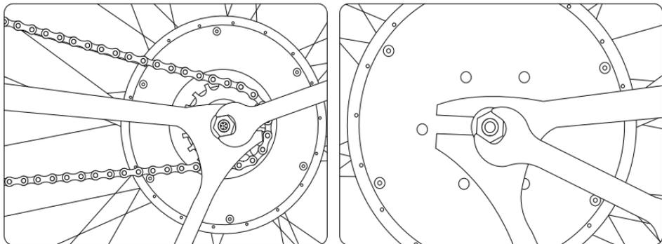
Tighten both M12 axle knots strongly.
