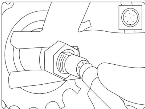
Carefully spin the charger in the socket and find the correct position in which the charger should gently fall into its place.
