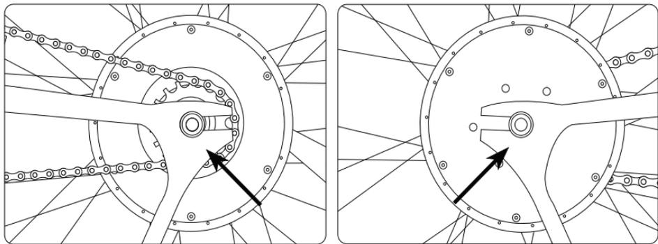
Screw on the axle covers onto the axle on both sides.
