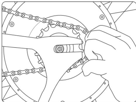
Place the chain on the sprocket.
